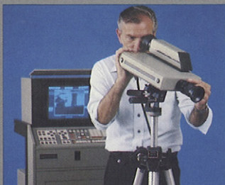
USE OF A SOLID-STATE VIDEO SENSOR DEVELOPED BY KODAK ALLOWS A VERY SMALL CAMERA TO PRODUCE UP TO 12,000 PICTURES PER SECOND.
