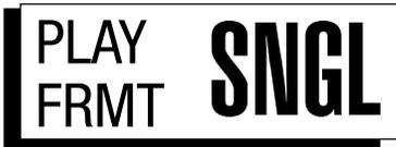
Press the **PLAY FRMT** softkey and then use the arrow keys to toggle between **SNGL** and **MULT**.
