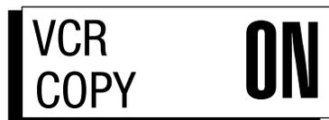
VCR COPY automatically downloads the pictures currently in memory to a VCR using the infrared control link to operate the VCR. When the playback is complete the Processor will stop the VCR, turn VCR COPY OFF and return control of the Motion Analyzer to the operator.
