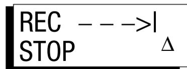
The Processor starts recording and continues to record until the STOP key is pressed.
