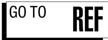
Press the **GO TO** softkey and then press any arrow key once to toggle between **REF** and **LAST**.
