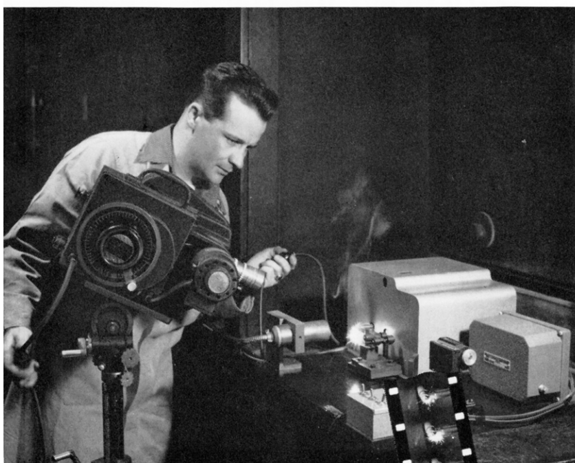
Above: Ready to film sparks produced by spark wheel testing machine. Note photoelectric cell, which has been adjusted to record only sparks of minimum acceptable intensity. Below: Close-up of sparking action. Speed of acceleration and rotation of spark wheel can be adjusted as desired.
