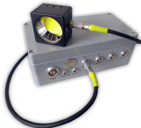
isCL-Box 4 CrashController 220 x 120 x 81 mm
