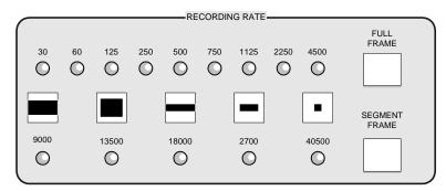
Press the Full Frame button to step through frame rates 4500 through 30. The LED just below the frame rate selected will illuminate. For example the LED below 4500 illuminates when the Imager is taking pictures at 4500 frames per second (fps). Pressing the Full Frame button will change the frame rate to the next lower setting until 30 fps is reached and then the next button press will return you to 4500 fps.
