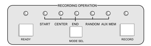
Press the Mode Sel (mode select) button to step through the various record modes from left to right. The LED under the operative record mode will be illuminated.
