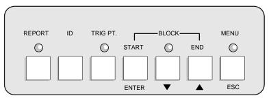
The Report function overlays the top and bottom of the image on the video monitor with text information. Press the Report button to toggle the display on or off. The information displayed is as follows:
