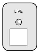
Press the Live button to place the Motion Analyzer in live mode. The LED above the button will illuminate to indicate that the processor is in live mode. Press the Live button again to take the processor out of live mode. The last image taken by the Imager will remain on the video monitor after live is turned off.
