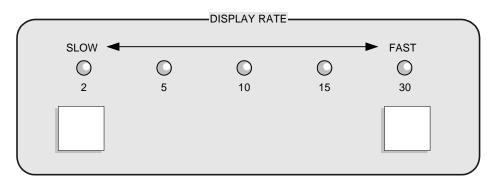
The one of five possible speeds in use is indicated by the illuminated LED. Press the button under the 2 to decrease the display rate. Press the button under the 30 to increase the display rate.
