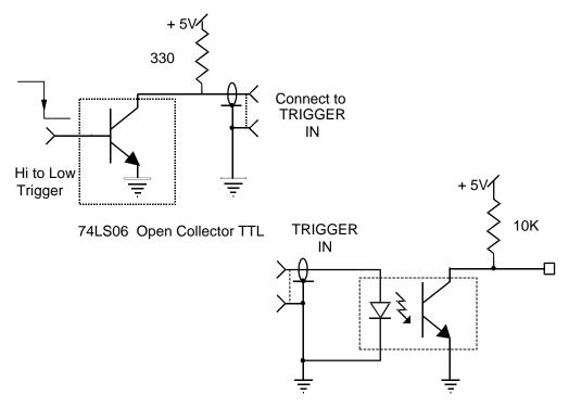
isolator requiring roughly 10 milliamps drive current from a 5 volt source. A simplified schematic for the input and a suggested driver are as follows:
